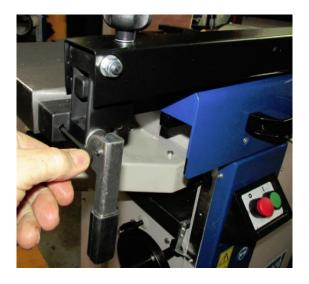
Now slide in the spindle guard extrusion (Shown as part 729 on page 37 of the factory manual) into the end of the cutter block cover arm but first fit the wear spring into the arm before sliding in the guard extrusion.
